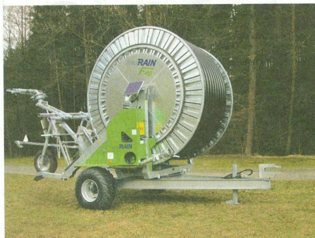
The Bauer ProRain reel irrigator comes in two models with a choice of six hose diameter/length configurations.
